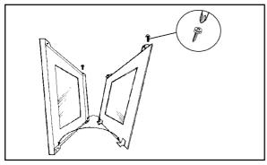
5. Clean the outer and inner glass using hot soapy water or Flash Cream cleaner may be used. DO NOT try to clean the aluminium foil which is inside the door. The foil is there to help keep the door cool, if it is damaged it will not work. Ensure that all parts are well rinsed and thoroughly dry before attempting to replace the outer door.
